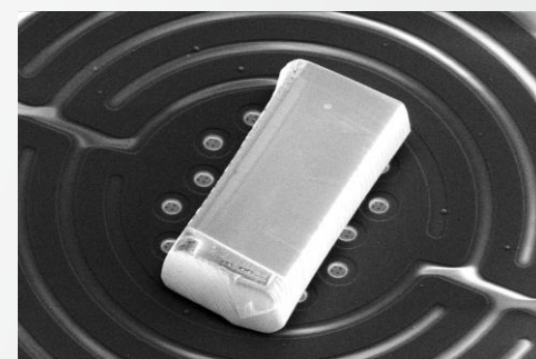
80μm x 35μm Ni superalloy chunk on MEMS chip.
